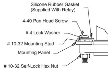
Non-Environmental Solder Termination Relay Sockets
